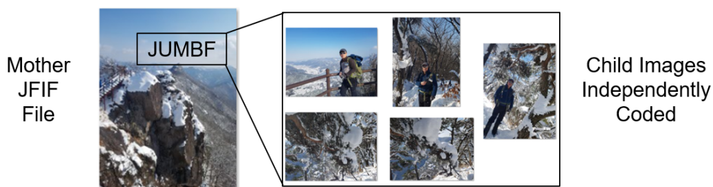
Figure 2 - Example of mother JFIF file embedding multiple child images independently coded
