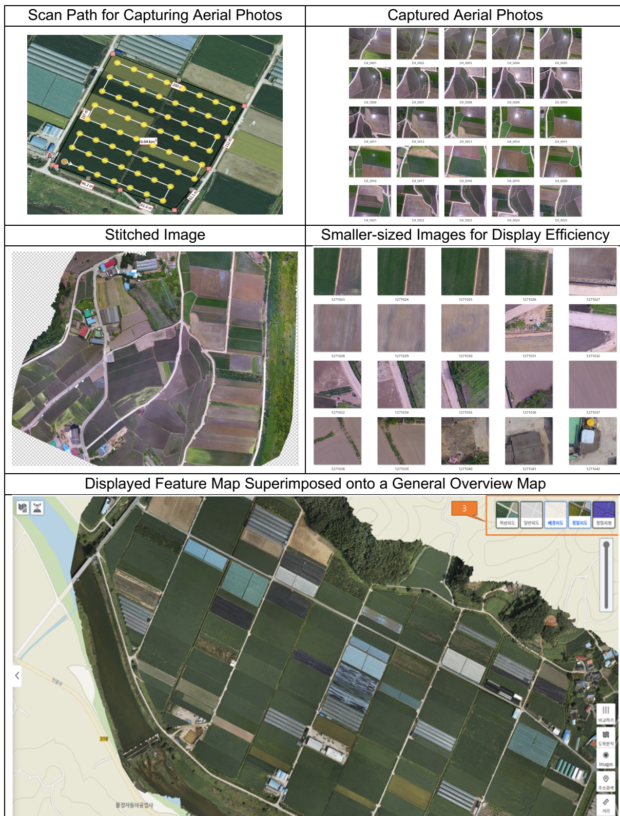
Figure 15 - Examples of drone images: captured aerial photos are used to form a larger stitched image which is then sub-divided to smaller images for displaying local regions superimposed with overview maps.
