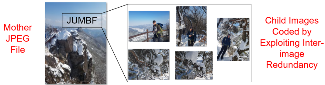
Figure 3 - Basic structure of mother JPEG file using JPEG GMIS
