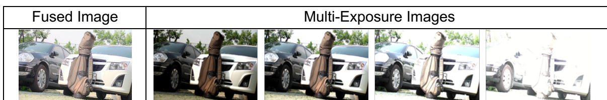
Figure 12 - Example of image set comprised of a single fused HDR image and multiple component images captured with different exposure times
