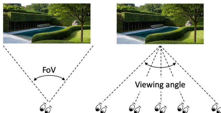
Figure 1 - Field of View (FoV) and viewing angle
