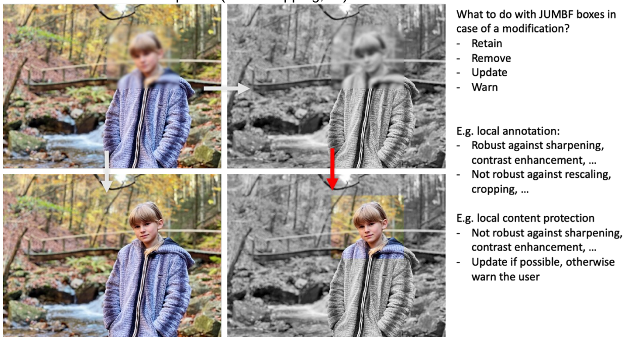
Figure 2: Illustrative example of an embedded Privacy & Security JUMBF box that needs to be updated in case a modification to the media asset content is made.
